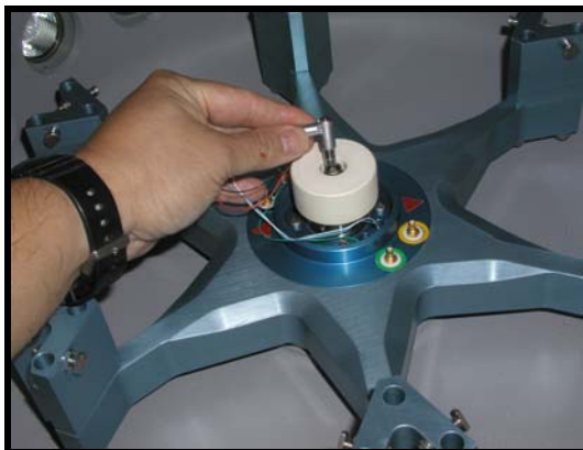
Connect temperature probe plug
