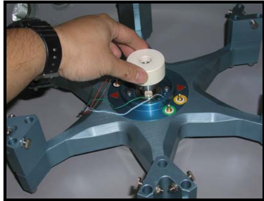
Secure rotor with locking nut
