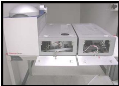
Photo 6 Cold trap and vacuum pump placement
