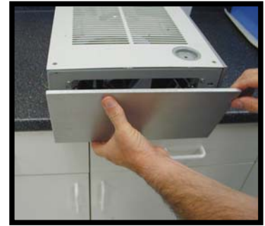
Photo 5 (Removing front panel from vacuum pump)
