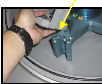
Insert Carriers (note insertion angle)
