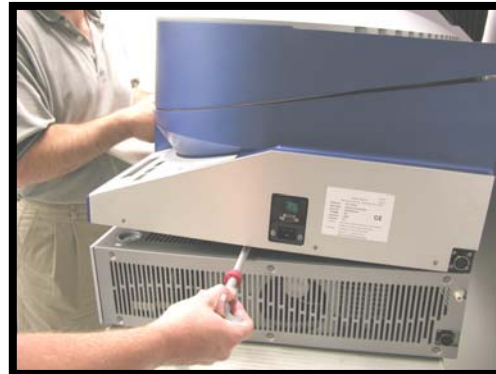
Photo 6e Removal of rolling pin
