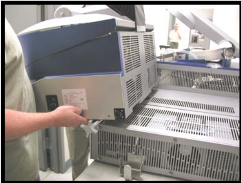
Photo 6d Position concentrator on rolling pin
