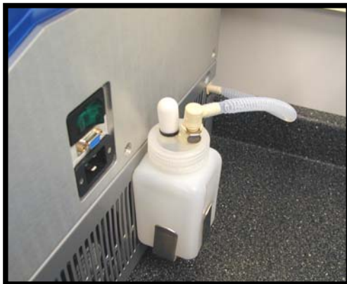
Photo Completed Post Trap assembly
