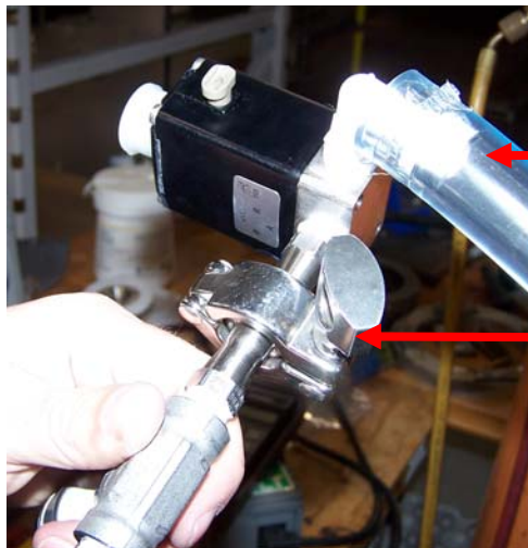
Fig EXP2.a-10 Connecting the 3 way valve to test fixture (P side adjustment)
